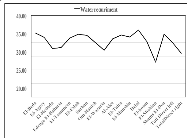
Fig 6: Actual water requirements of Dakalt canal
